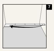
To begin the second row, use the remainder of the cut plank you used to finish the first row.
