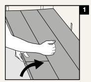
When a plank is locked, it is not possible to dismantle it by hand. Lifting up and knocking gently on a plank will unlock the row — fold up to fully release the long side.
