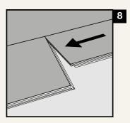
Position the second plank to the right short side of the first plank.
