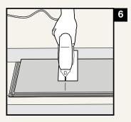
Cut the row's last plank to size. If you are using a jigsaw, cut it face down. If you are using a hand saw, cut it face up.
