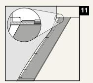
The first and last row may need to be adjusted if the wall is uneven. To achieve this, trace the wall profile to the first or last plank, cut, and install.
