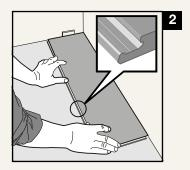
Now it's time to lay the first plank in the first row. Start in a left corner and lay a plank with the tongue side facing the wall. Now insert a wedge between the wall and the plank's left short side so there is a gap at least ½" (8-10mm) wide.
