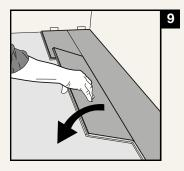
Fold down the second plank, making sure it's positioned tightly to the first plank — press down firmly and listen for the click that means it's locked in place.
