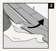
Once the whole long side is released each plank can be dismantled by angling the short sides up vertically.
