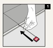
Position the dismantling tool into the gap between the tongue and groove on the short end of the plank. Push the dismantling tool into the short side.
