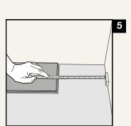
Continue installing the first row. When you are close to the wall on the right side, place a wedge at the wall and measure the length to determine the size of the row's last plank.
