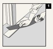
Door frames can be removed and raised, but it's usually easier to cut them. Use a loose plank as a template and saw off the excess. Ensure that the floor is not pressed between the subfloor and the door frame.
