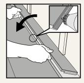
Remove the locking element/hook as shown in the diagram. Use white PVAc glue to connect the planks. Press/place wedges between the glued strip and the wall.
