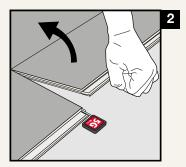
The short side should now be unlocked and the plank can be lifted.
