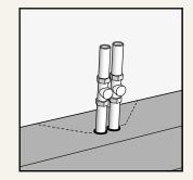
Mark the center point of the pipes on the plank. If the required expansion gap is 10mm, drill holes 20mm bigger than the pipe diameter. Cut as shown below. Apply white glue and install the floor pieces. Cover the holes with pipe collars or fill with a joint sealer.
