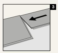
Position the second plank to the right short side of the first plank.
