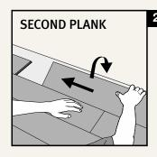
Angle the long side groove of the second plank into position at the tongue of the adjacent plank from the previous row and fold down. Now slide the second plank to the left to position it to the right short side of the first plank. Press down firmly and listen for the click that means it's locked in place.
