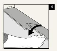
Fold down the second plank, making sure it's positioned tightly to the first plank — press down firmly and listen for the click that means it's locked in place.
