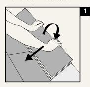
When installing in reverse, start from the left. Angle the long side groove into position at the tongue of the adjacent plank from the previous row and fold down to lock into place.
