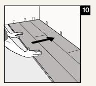
Continue to install the row as before. When you have completed 2-3 rows insert wedges between the wall and the first row so there is a gap at least  $\frac{1}{2}$ " (8-10mm) wide.
